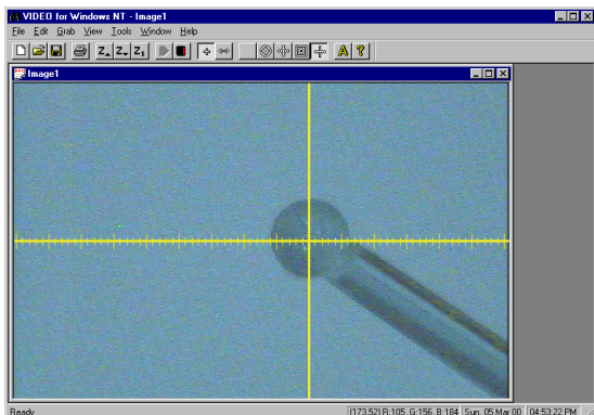
Figure 4-24. Crystal centered on crosshairs ( \phi = 0^\circ )
