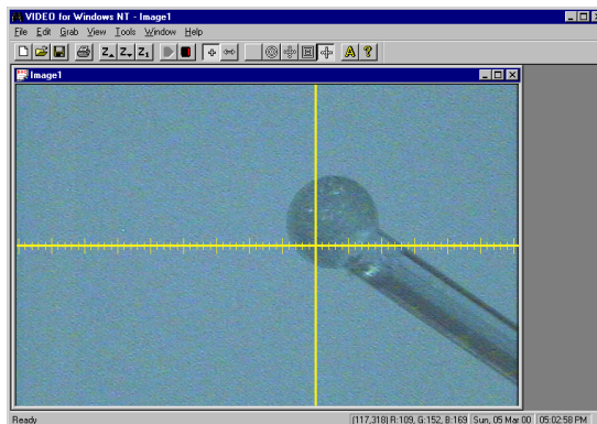
Figure 4-25. Crystal oriented for Y-axis adjustment
