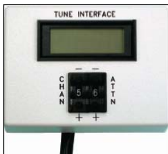
Figure 7 TUNE INTERFACE remote
