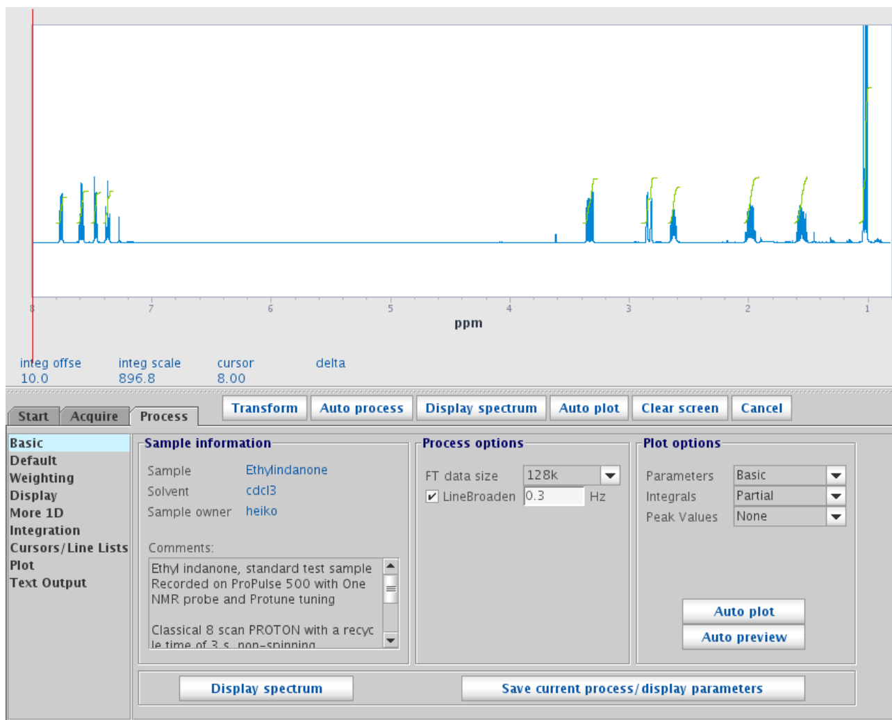
Figure 78 The Basic parameter page for a 1D data set
